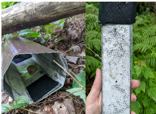
Track tube (left) and associated track plate with footprints of small mammals.
